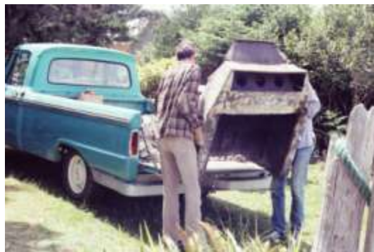
Steve and Dave load the old "Heatalator" into Dave's pickup truck. The Heatalator has rusted out completely, and instead of sending warmed air into the cabin, it sent smoke and soot.
